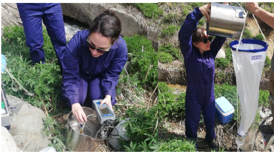
Image 8. River sampling for microplastic detection.
