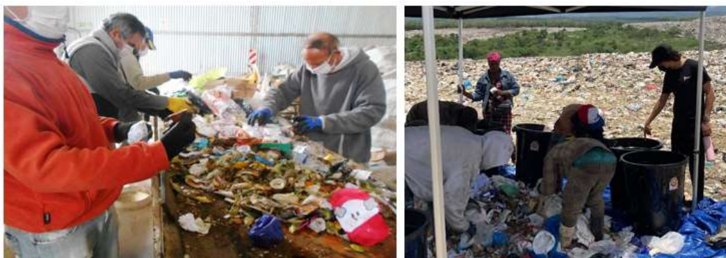
Figure 7: Example of waste characterization activities conducted by INTI in Argentina (left) and by adelphi in Dominican Republic (right)
